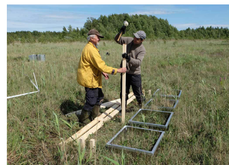
Installation of chambers for the measurement of greenhouse gases in the predecessor project LIFE Peat Restore.
